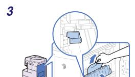
Pull down the upper cover of the fixing unit by the tab, and remove any jammed paper.
